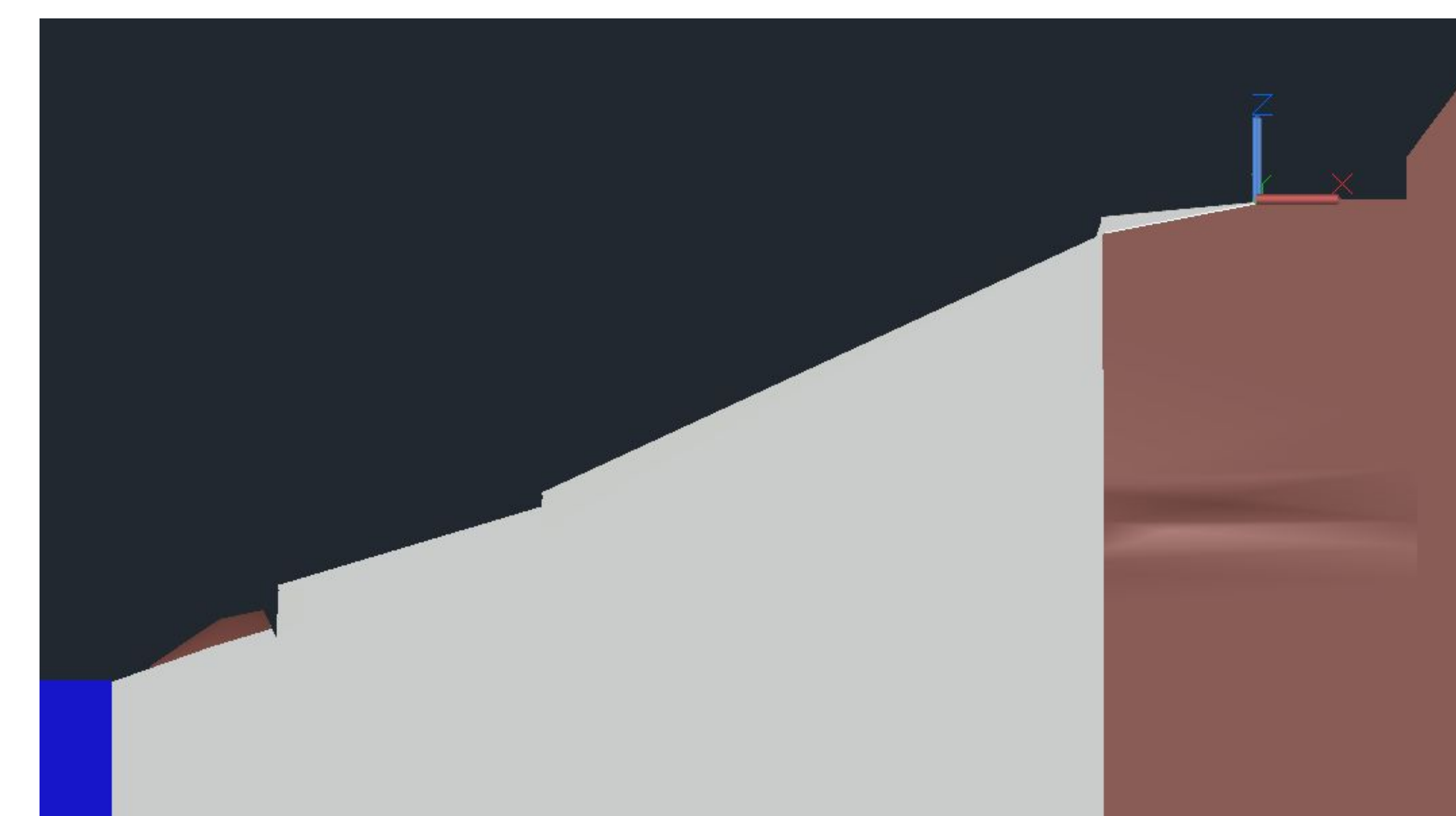
Figure 7 CAD Model of Crib Wall and Gabion Basket design Wall Dimensions (from high elevation to low): Log wall - 5x3x36 ft Gabion wall middle - 4x2x36 ft Base Gabion - 6x3x36 ft
